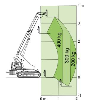
The Handler 400's maximum load capacity with the boom retracted amounts to 400 kg (including the fork attachment).
