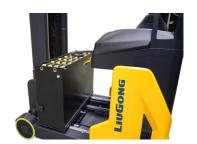
In order to replace the battery its tray should be reached forw ards. The mechanism for battery's tray release is located near with operator's foot.
