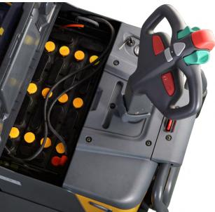
Long operating time through high capacity with 3PZS battery.
