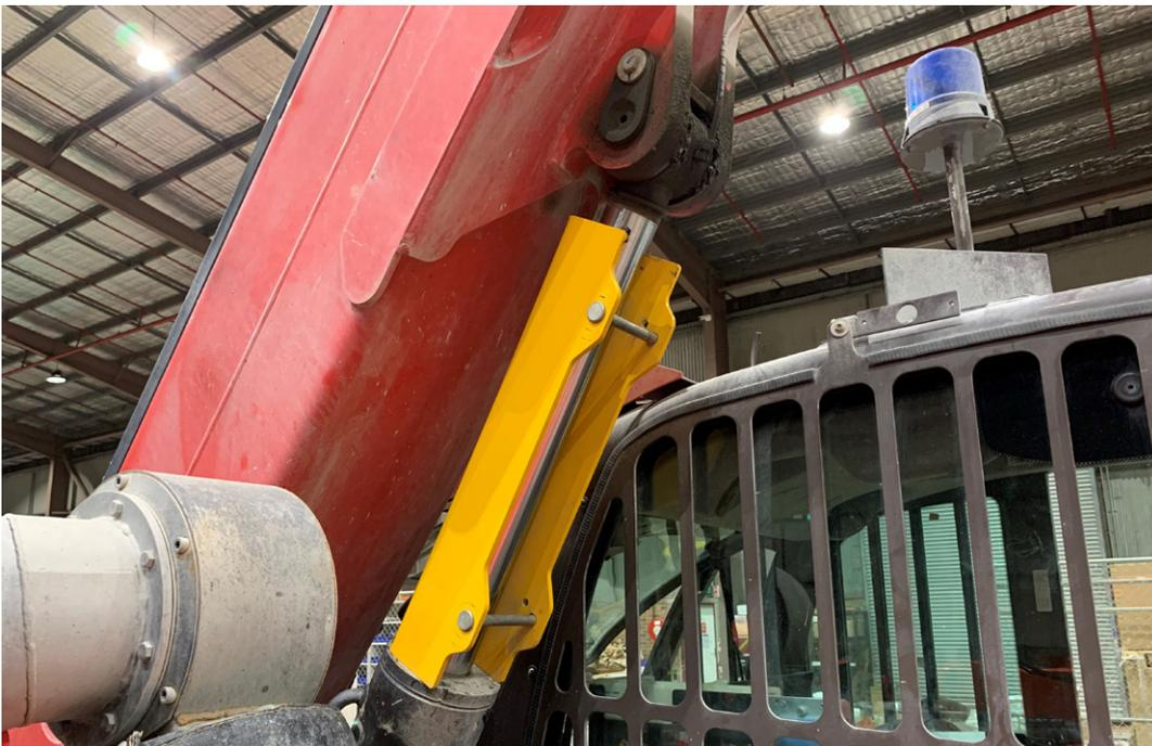
**Figure 15: Always install the safety prop when working under the booms**
