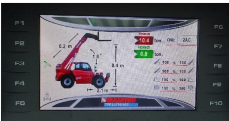
Figure 6: Typical boom length indicator (electronic)
