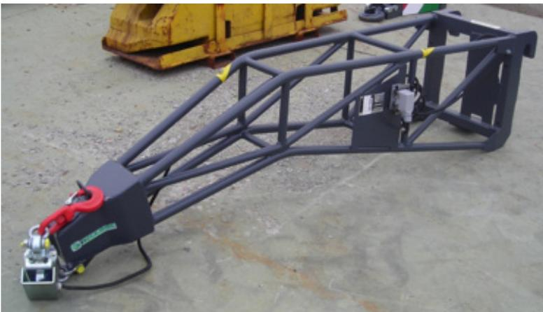
**Figure 13: Roof-truss jib**
