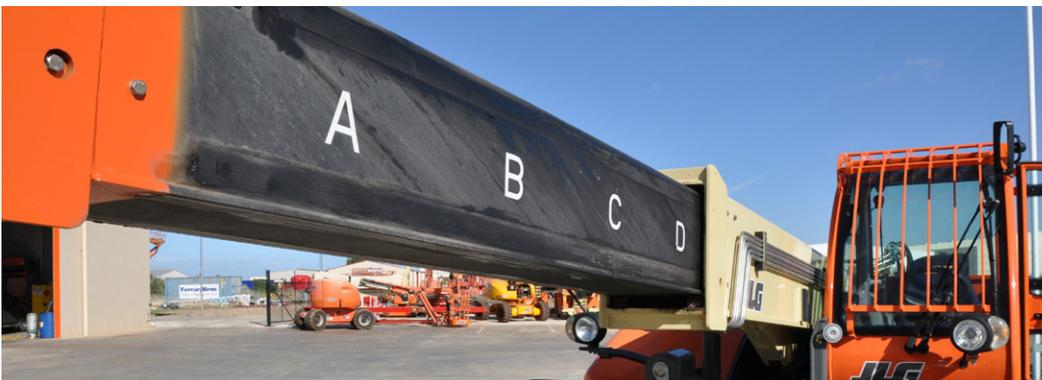
Figure 5: Typical boom length indicator (mechanical)
