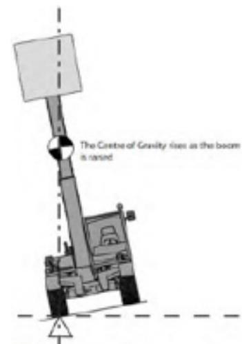
It is important to consider the telehandler stability in three configurations – longitudinal (forwards stability), lateral (side stability) and rearward stability.
