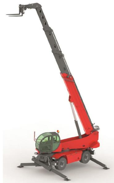
Figure 4: Typical slewing telehandler
