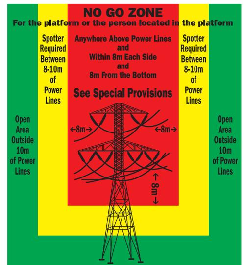
Note: If the boom is insulated and has a current test certificate issued by a NATA approved laboratory, no spotter is required in the yellow area. The 3.0m clearance is from the top of the bucket of the elevating work platform.
