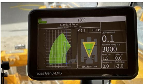
**Figure 10: Typical actual capacity indicator**
