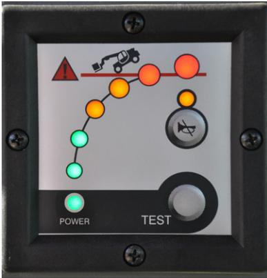
**Figure 9: Typical longitudinal load moment indicator**
