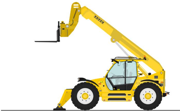
Figure 3: Typical non-slewing telehandler
