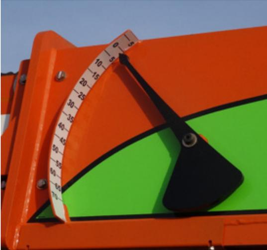
**Figure 7: Typical boom angle indicator (mechanical)**
